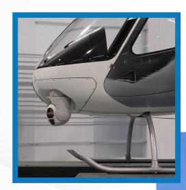
Certified by the Manufacturer as part of the helicopter, this device will allow easy integration of a wide range of sensors and cameras to fit your specific mission (gimbal, lidar, stinger etc.).
