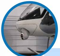
Certified by the Manufacturer as part of the helicopter, this device will allow easy integration of a wide range of sensors and cameras to fit your specific mission (gimbal, lidar, stinger etc.).
