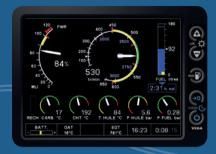
The heart of the avionics is the EPM, a dedicated multi-function display monitoring 36 parameters and providing advanced functions such as:
